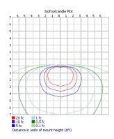
Recommended for undivided tunnels where equal lumens are with and against traffic flow.
